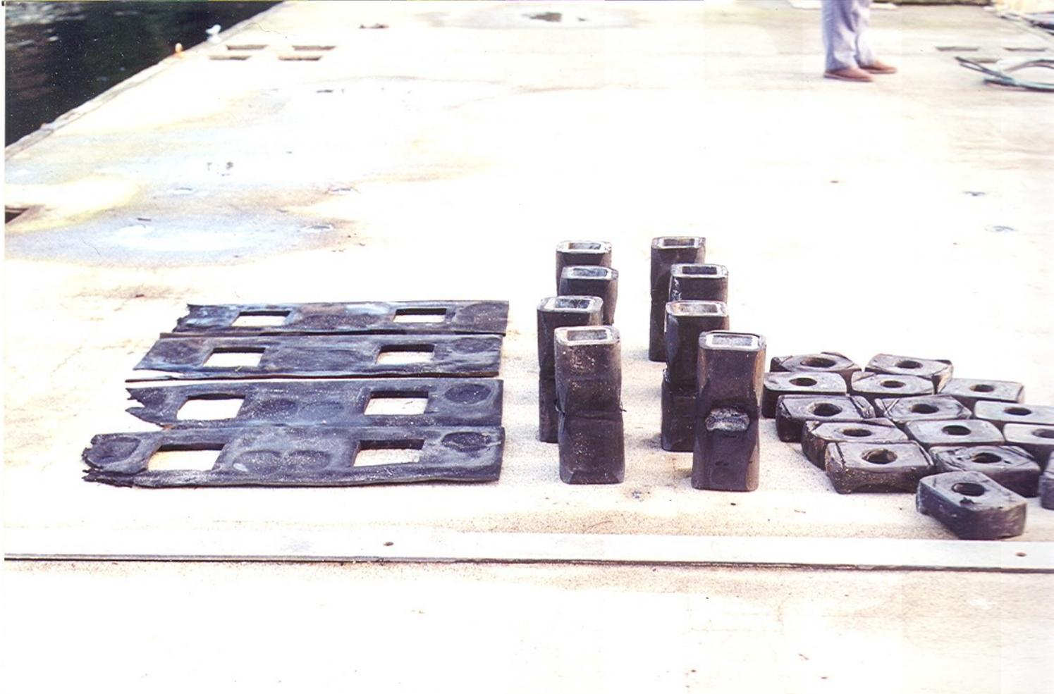
*A worn-out set of connector hardware for the original sections of A Dock. These are the buffer pads between the sections on the left, the shear connectors in the centre, and the bolt bumpers on the right. They have been lasting approximately 15 years and were replaced by a work party in less than a day.*
